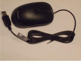
**USB mouse** - the mouse should be connected to the USB port **before** turning on the computer.
