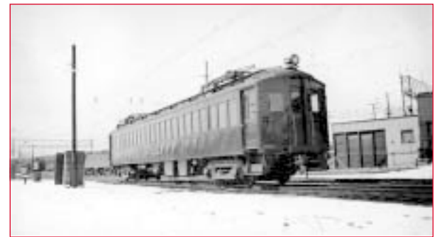
New Haven Railroad AC-only multiple unit motorcar 4060, in Stamford, CT, 1936
