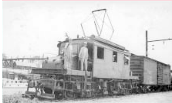
New Haven Railroad electric engine switcher number 0200, engine type B+B, with raised pantograph, in Stamford, CT, 1935
